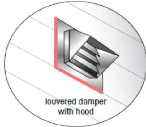
Depiction of typical external damper assembly
